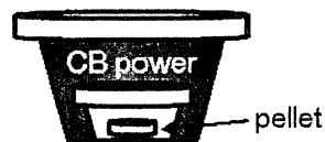
Fig. 1 Reduction heating by double-crucible method.
