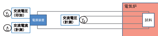
Fig.2 Schematic measurements of hot electrical resistivity.
