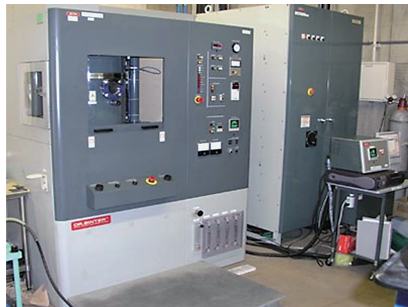
Fig.1 Apparatus of spark plasma sintering.
